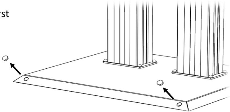
2. The base can now be fixed to the floor using fixings up to 8mm in size.
