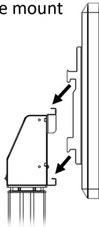
3. Secure the screen in place using the clips and two M6\*50mm bolts with washers.
